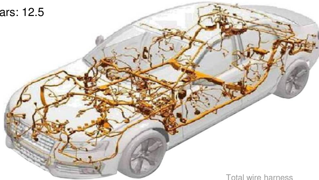
Total wire harness in modern vehicle
