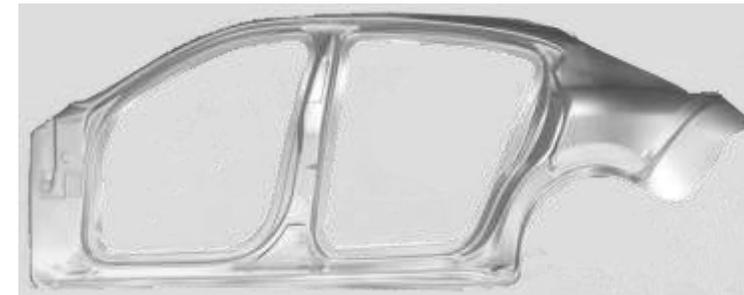
Press trial with HA 6016-X on die designed for steel, radii changed for aluminium
